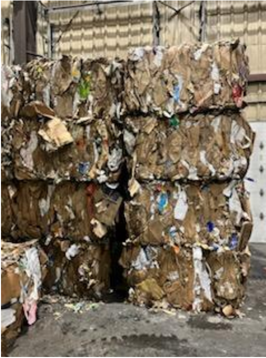
Photo 1: Old Corrugated Cardboard (OCC), Side View
